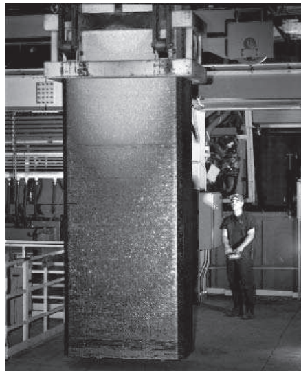
Fig. 3.11. Large titanium slab directly cast from a cold hearth melting furnace (courtesy Teledyne Allvac)
