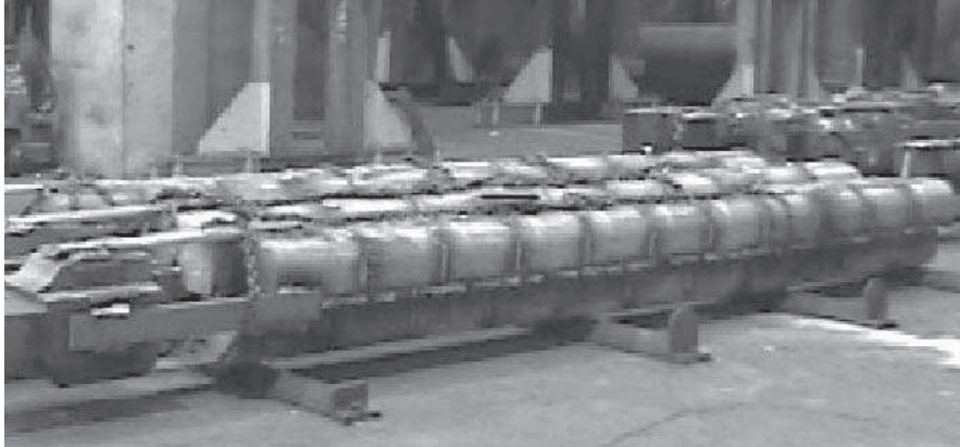
Fig. 3.6. First melt VAR electrode with welded individual briquettes and the stub on the left (courtesy RMI)
