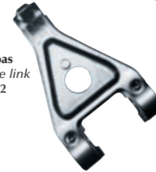
Tige coulissante train central CLG sliding member 300 M 1670 kg
