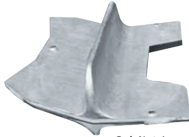
Croix Vert. Ar. Central wing box vertical fitting 7010 214 kg
