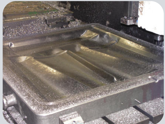
Mould for military engine exhaust outlet
