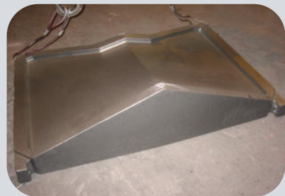
Tooling for Jet flap or windshield front fairing of airplane
