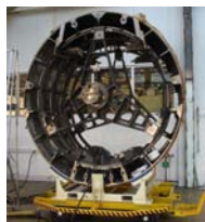
Tooling for composite inlet of A380 engine
