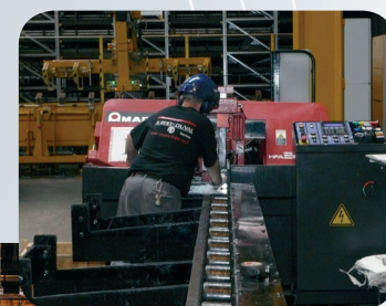
A set of saws able to cut bundles of all alloys.
