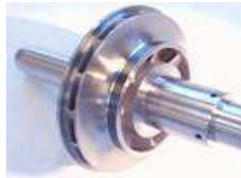
TA6V impeller for space rocket
