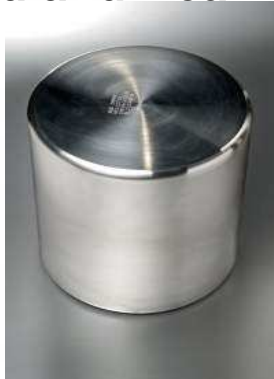
N18 billets for the production of turbine discs by isothermal forging
