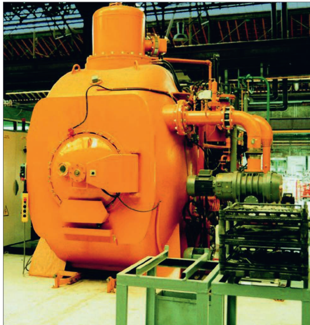
Low pressure carburizing furnace at Aubert & Duval
