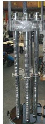
Ball screw (THSA) for the A380
