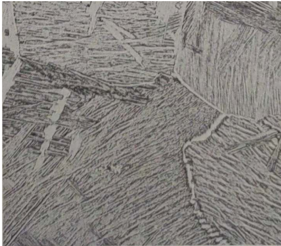
2 HF, 8 HNO 3 , 90 H 2 O 200× 2710 Ti-6Al-4V extrusion, heated for ½ hr at 1850 F (1010 C), air cooled, then heated for 1 hr at 1250 F (677 C), air cooled. Structure: acicular alpha (transformed beta); alpha at prior beta grain boundaries.
