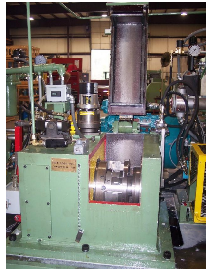
An automatic compensating head on a rotary wire shaver for diameters up to 1.496" (38 mm)
