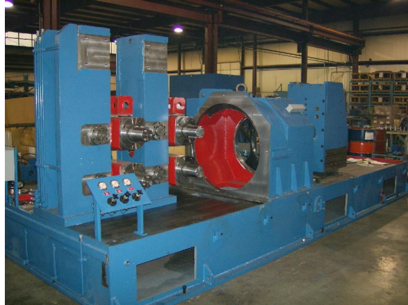
The 200mm turner machine base, with major components, ready for fastening to the base. (Spindle not in turning head housing.)
