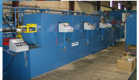
A rotary coil shaving and polishing system for high strength stainless and super alloys up to 1.250" (32 mm)
