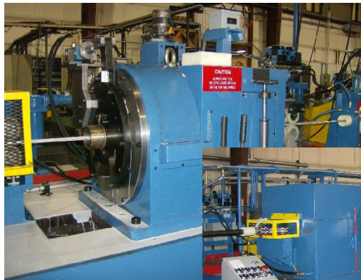
A rotary coil shaving and polishing system for high strength stainless and super alloys up to 1.250" (32 mm)
