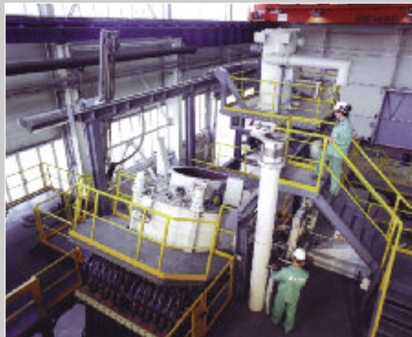
Melting chamber in pouring position
