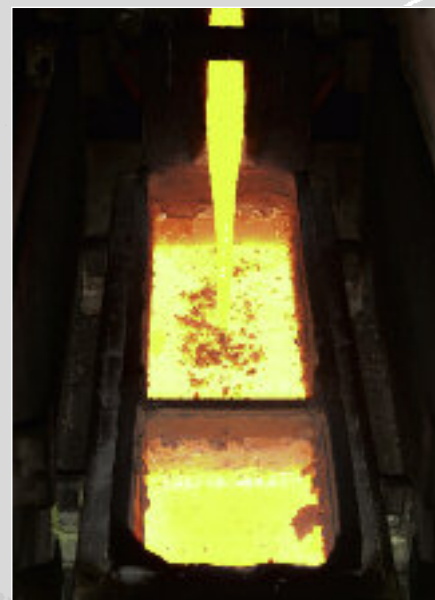
Tundish box with slag weir
