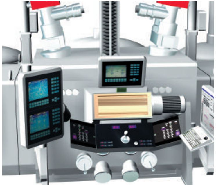
Operator's cockpit at an EB/PVD-production coater
