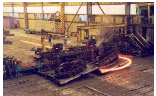
Bar and wire mill
