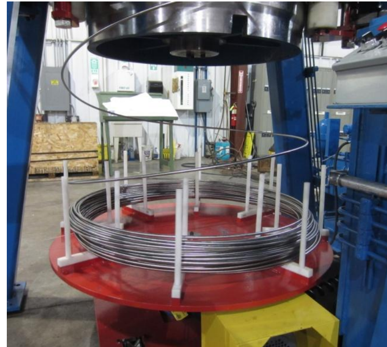
Drawn coil is being cast between the fingers of the take-up carrier
