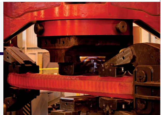
UKAD state-of-the-art facility with 4,500 ton forging press and lean manufacturing environment
