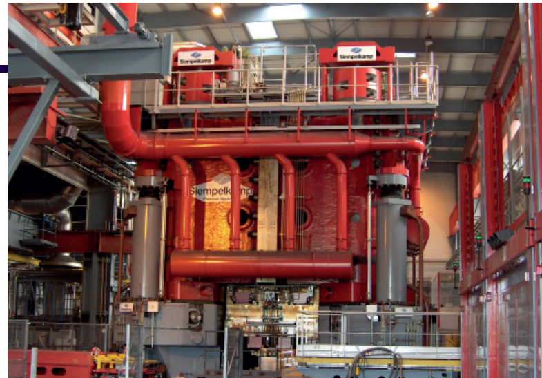
Aubert & Duval's 40,000 metric ton closed die forging press
