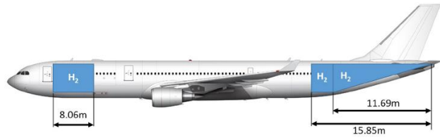
Figure 21 : H 2 tank layout for A330 aircraft.
