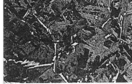
(f) Typical Microstructure of Overheated Material at 100X
