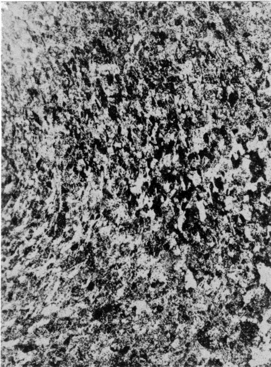
FIGURE 4 - LEVEL 40 TITANIUM BILLET MACROSTRUCTURE AT 1X MAGNIFICATION
