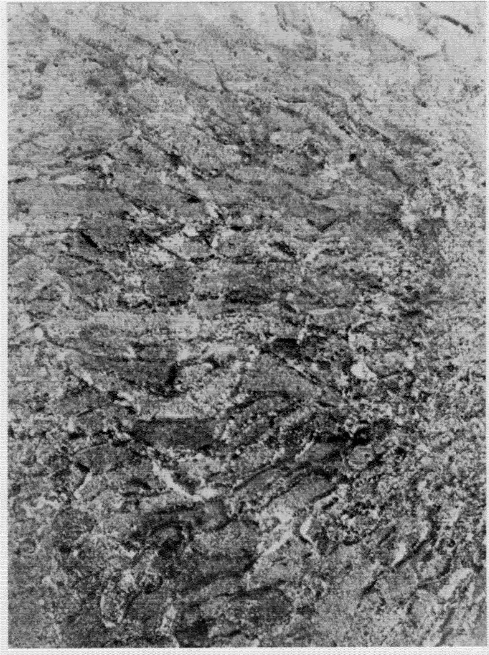
FIGURE 9 - LEVEL 90 TITANIUM BILLET MACROSTRUCTURE AT 1X MAGNIFICATION
