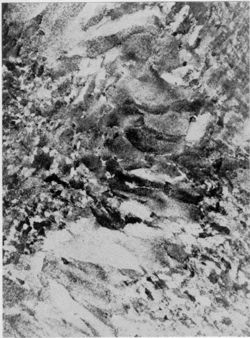
FIGURE 10 - LEVEL 100 TITANIUM BILLET MACROSTRUCTURE AT 1X MAGNIFICATION
