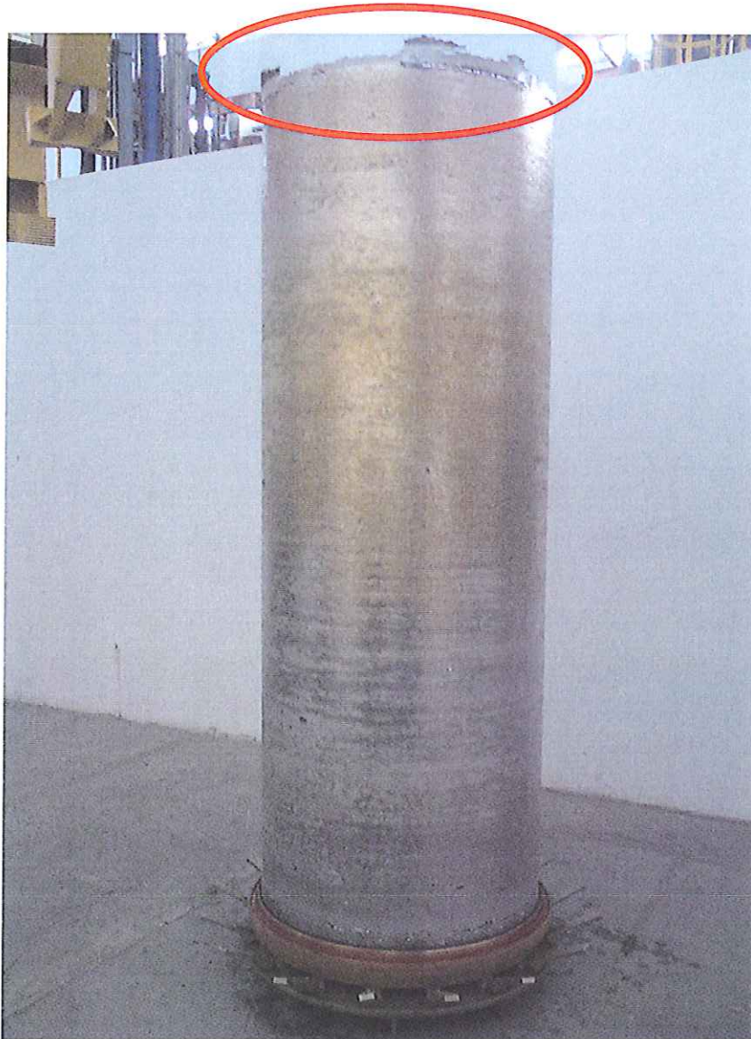
Figure 2 - unacceptable: top with crown (acceptable surface)
