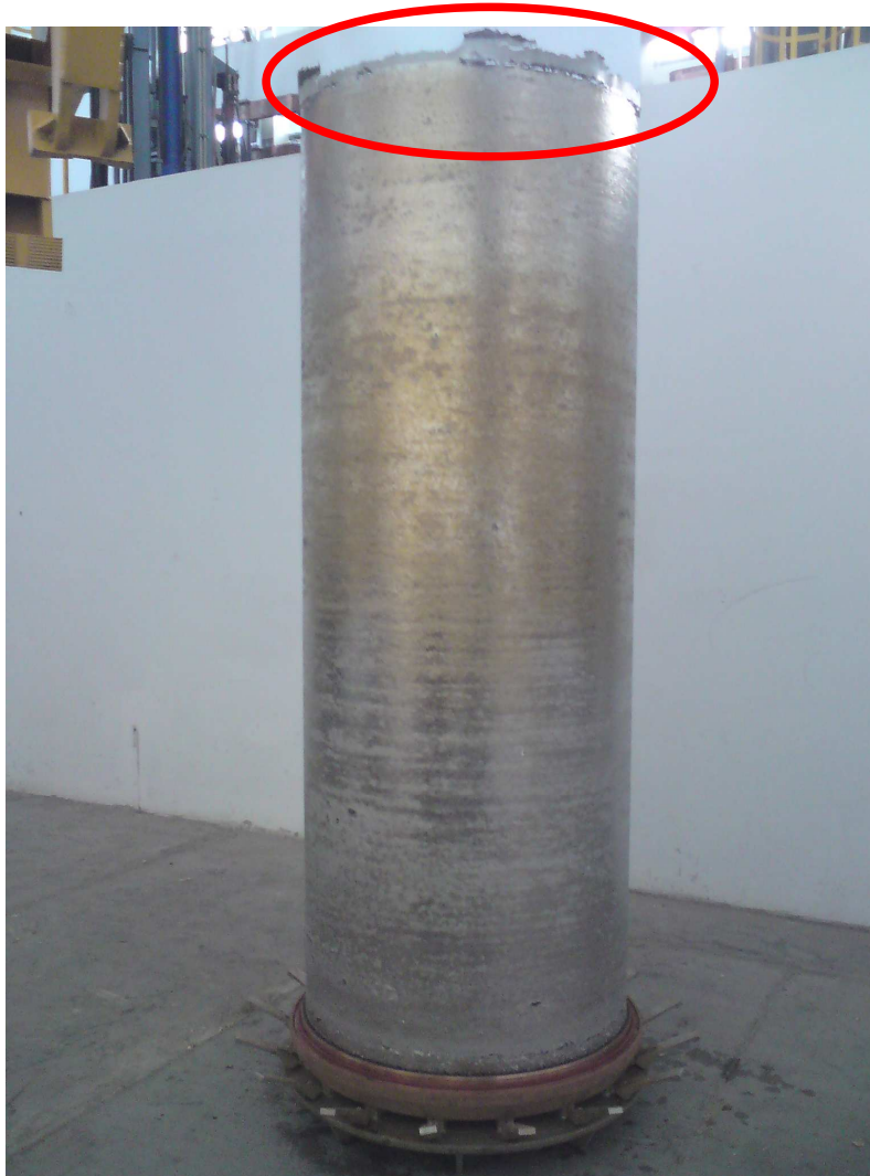
Figure 2 - unacceptable: top with crown (acceptable surface)
