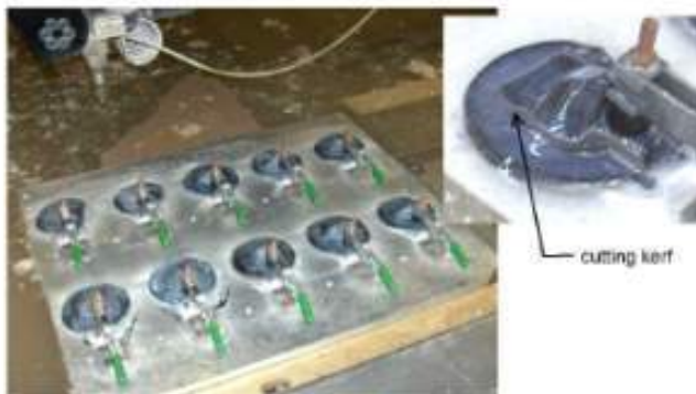
Flash removing by water jet cutting
